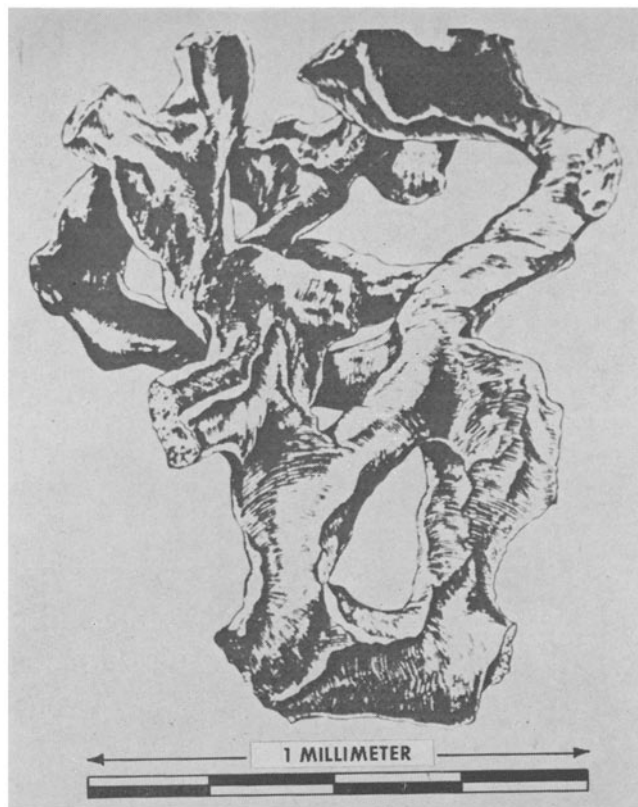
Fig. 2. Metallic cast of pore spaces in a consolidated sand.
